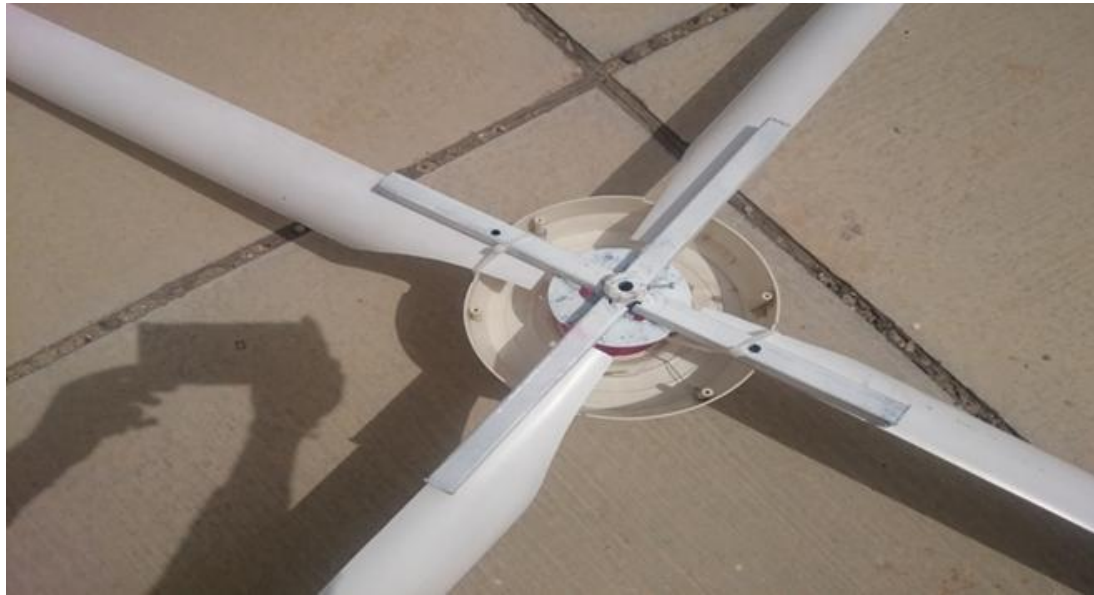
The turbine blade base
